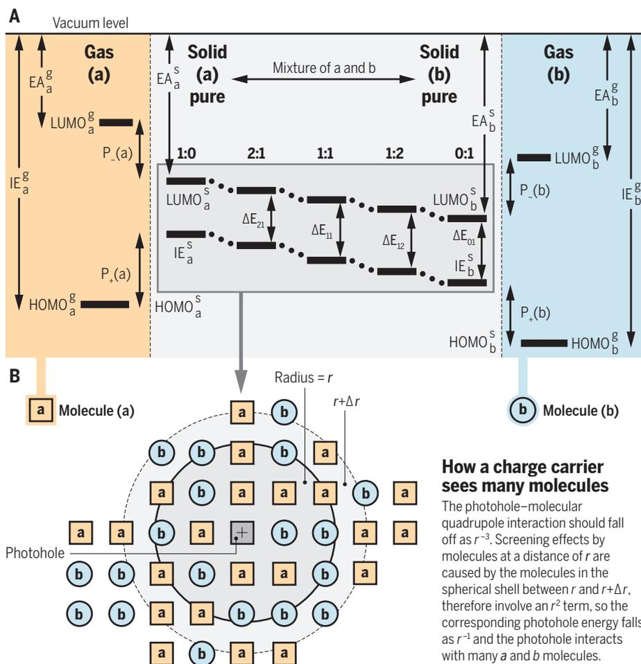
**Smooth changes.** (A) Schwarze *et al.* found that mixtures of organic semiconductor molecules, 1 and 2, change their electron affinities (EA) and ionization energies (IE) smoothly; the solid-state values are offset by polarization terms. (B) The origin of this smooth change can be explained by considering a photogenerated charge carrier. It interacts with the quadrupole moment of many nearby molecules, sampling a population of both 1 and 2.
